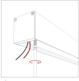
A Run the wires through the hole, then secure the fixture into the surface.
