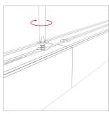
2 Drill in the connection piece where both fixtures connect.
