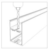
Drill a hole into the fixture for low voltage
