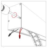
Secure the end caps and install the LED strip on the fixture surface
