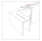
2 Put the connector into the Profile.
