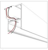
4 | Place the power supply inside the fixture and connect the electrical wires
