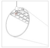
5 Install the suspending system and connect the electrical wires.
