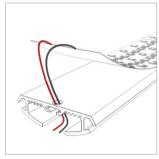
3 | Install the LED strip on the fixture surface.
