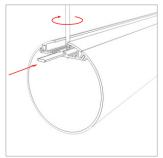
Install the two fixtures together using a connection piece.
