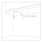
Make the electrical connection to the power supply and then run the wires to the location of the light fixture.
