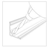
2 Drill a hole into the fixture for low voltage
