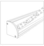
4 Install the LED strip on the fixture surface.
