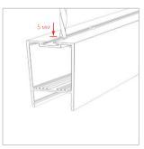
Drill a hole into the fixture for cover the screw, keep it in the same level with the Profile, and the depth of hole is less than 5mm.
