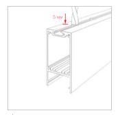
Drill a hole into the fixture for the screw, keep it in the same level with the Profile, and the depth of hole is less than 5 mm.
