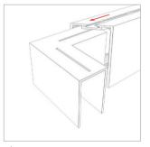
2 Put the connector into the Profile.
