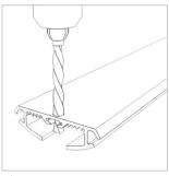
2 Drill a hole into the fixture for low voltage wires.
