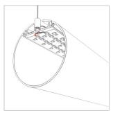
5 Install the suspending system and connect the electrical wires.
