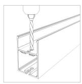
2 Drill a hole into the fixture for low voltage
