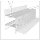
Drill a hole into the fixture for low voltage wires and for mounting brackets.
