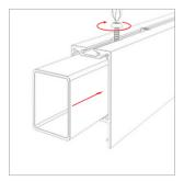
2 Put the connector into the Profile then fix with screw.
