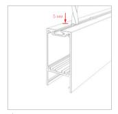
Drill a hole into the fixture for the screw, keep it in the same level with the Profile, and the depth of hole is less than 5 mm.
