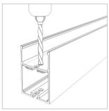
Drill a hole into the fixture for low voltage wires
