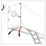
5 Secure the end caps and install the LED strip on the fixture surface.
