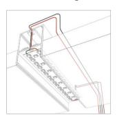
Electrical connection must be made from both sides for fixtures longer than 2500mm.
