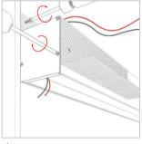
4 Secure the end caps and fix the luminaire on the wall, run the wires through the hole.
