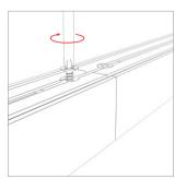
2 Drill in the connection piece where both fixtures connect.
